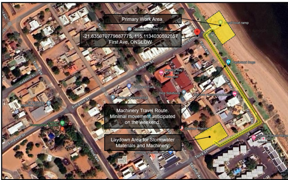
Figure 2 – Primary work area and laydown area
